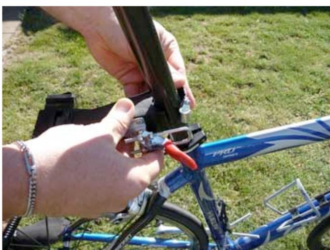
Close the clamp and test the grip tension. Adjust the outer nuts on the U-piece until a satisfactory grip is obtained.
