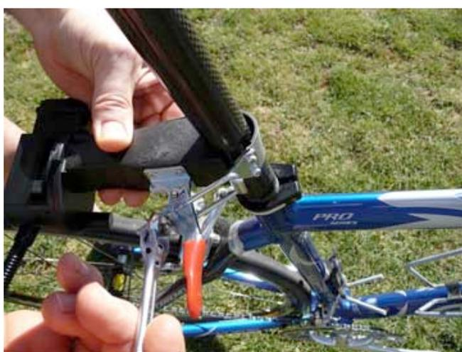
Check that the wand rotates smoothly and the rotation clip operates correctly at the horizontal position.
